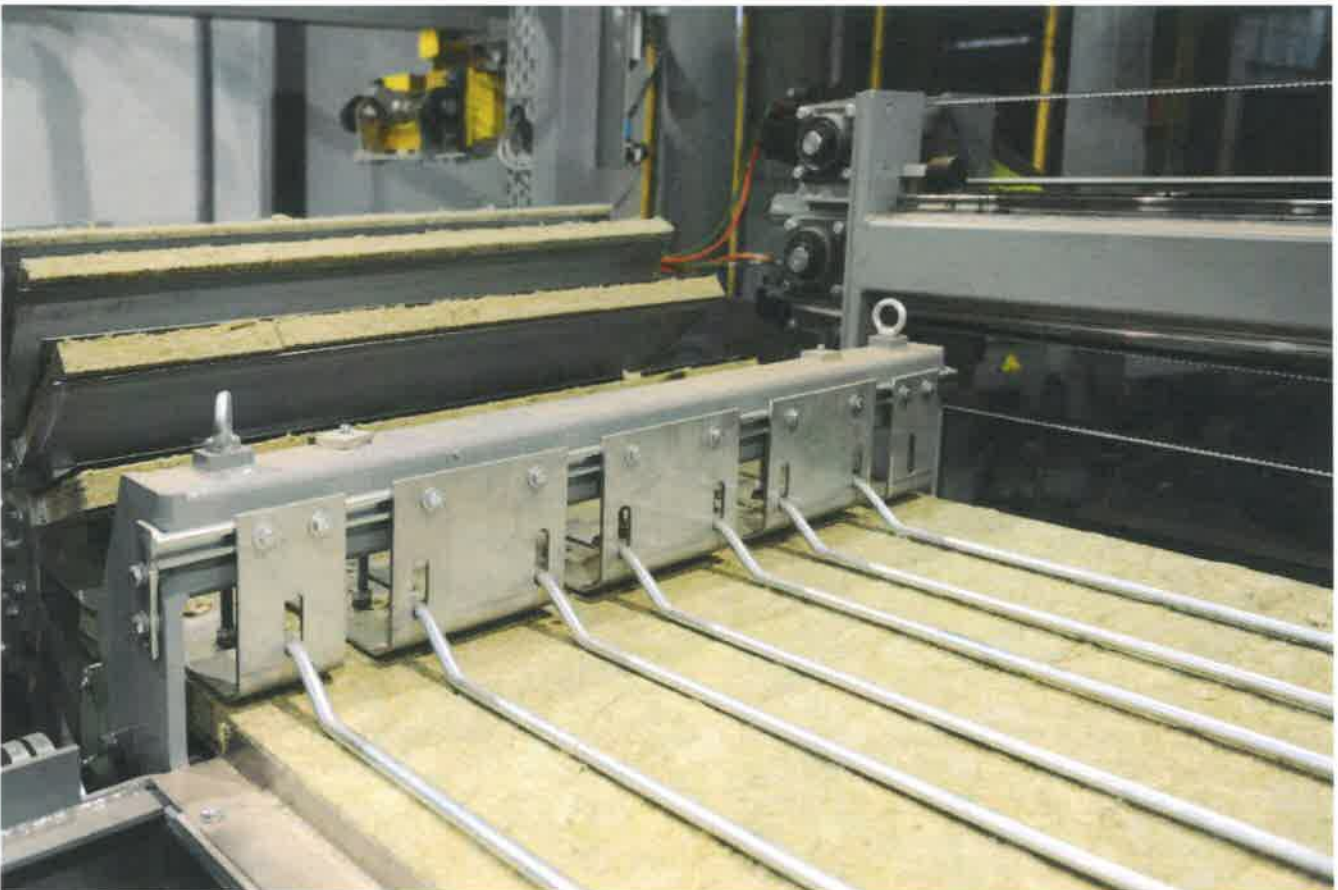
Photo 2 - Thermal insulating pads prepared at carousel
