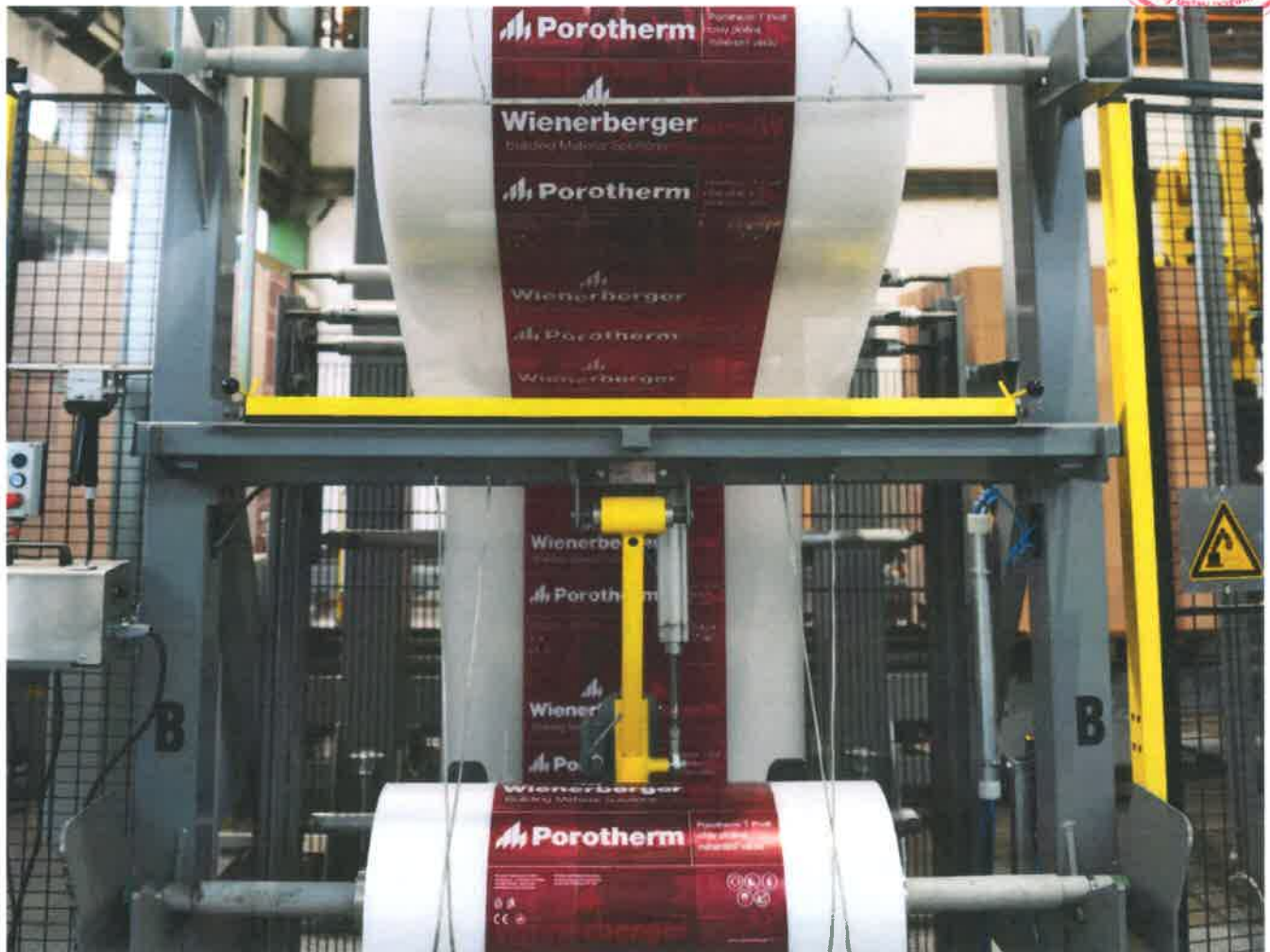
Photo 6 - Foil wrapping line for packing of pallets with finished products
