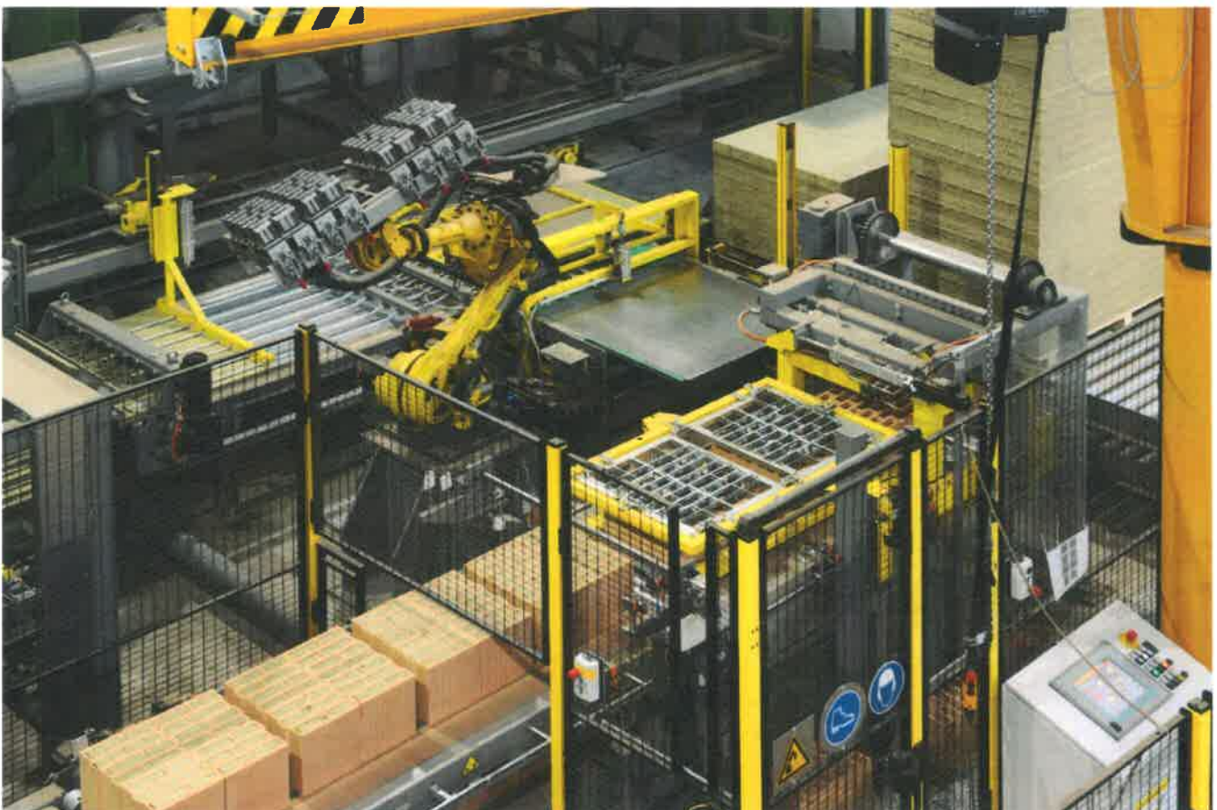
Photo 4 - Inserting thermal insulation into brick blocks
