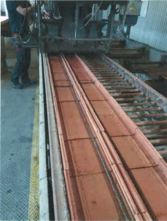
Photo 2 – Moistured U-shaped masonry units before concrete placement
