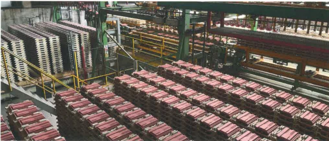
7 | Loading kiln cars
