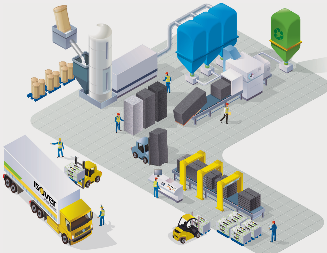
Fig. 3 – Manufacturing process schema
