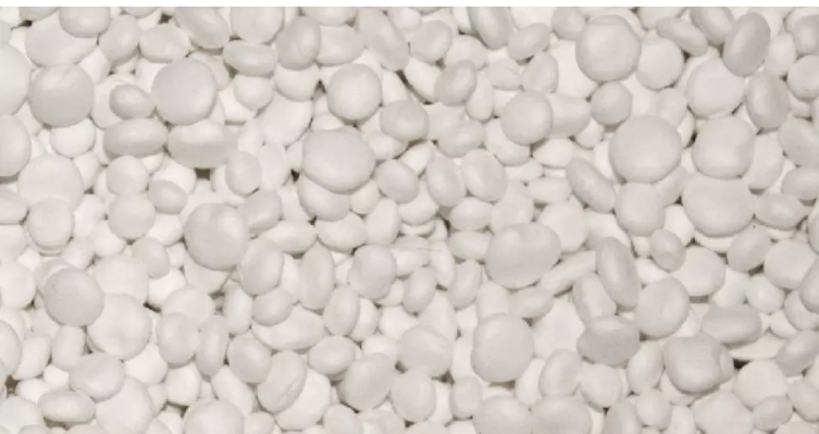
Fig. 13 - Raw material for the production of EPS
