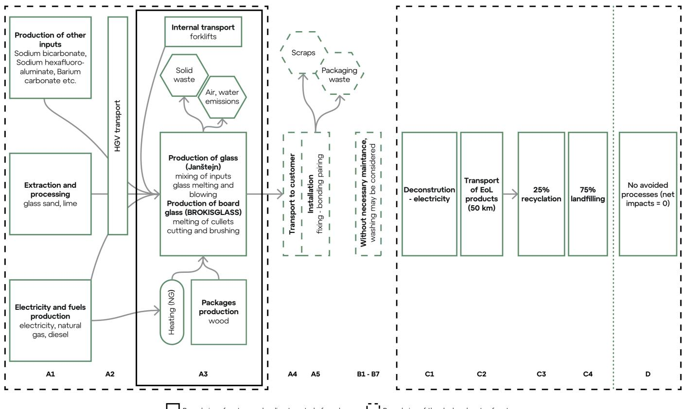
Boundaries of system under direct control of producer
